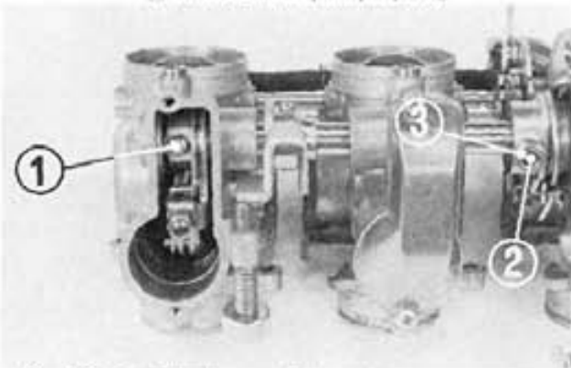
Fig. K7-6 ① Link arm fixing screw ② Set screw ③ Lock nut
