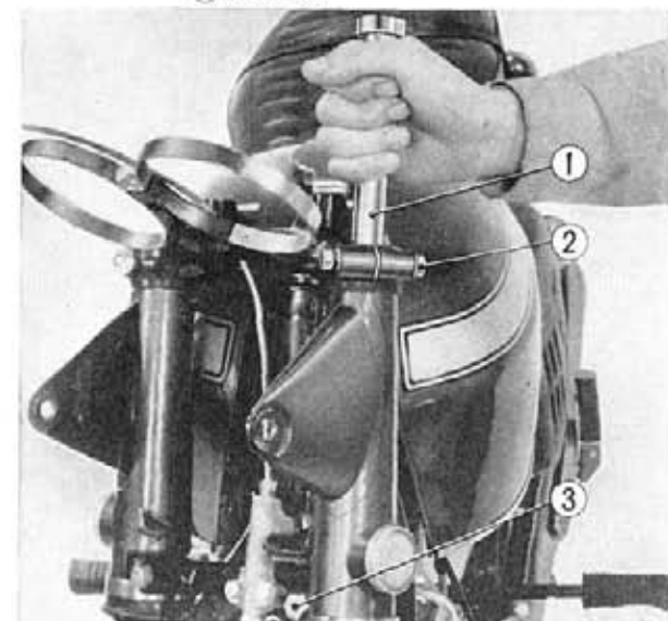
Fig. 11-20 ① Front fork assembling bar ② Front fork pipe setting bolt (8 mm) ③ Front fork pipe setting bolt (10 mm)
