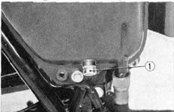
Fig. 15-7 ① Oil tank drain plug
