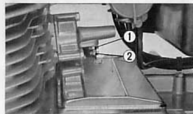
① Lock nut ② Tensioner lock bolt
