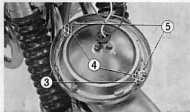
③ Lock pins ④ Lock screws ⑤ Sealed beam unit retaining screws
