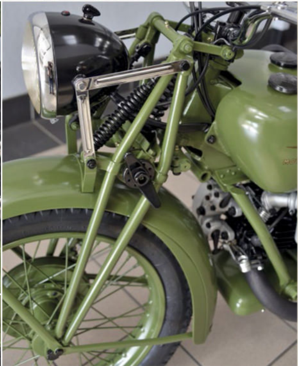
ABOVE Ruggedly constructed girder fork controls front end.
