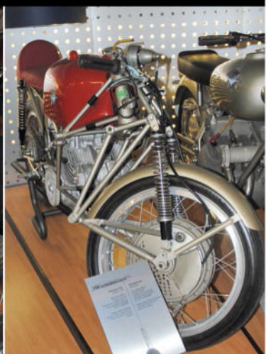
ABOVE Prototype 350cc DOHC twin cylinder racer from 1955 produced 46.5 horsepower at 12,000 rpm.
