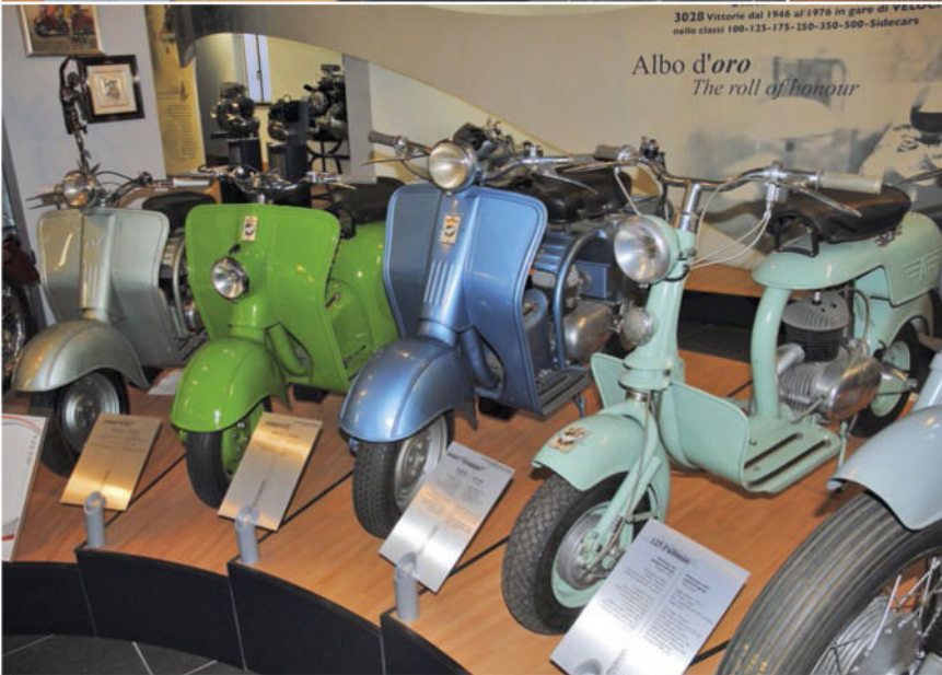
Colourful line up of MV scooters, ranging from 1948 to the light blue 1952 Ovunque ("Everywhere") on the right. All featured swinging arm rear suspension with 4-speed gearboxes.
