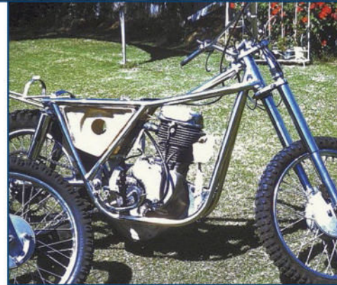
ABOVE Dave Basham on the ESO leads Peter Heywood at Snake Gully track, SA. BELOW The engine from Dave Basham's original ESO installed in a Metisse-style frame built by Don Pretjohn. (Photos from Peter Heywood)
