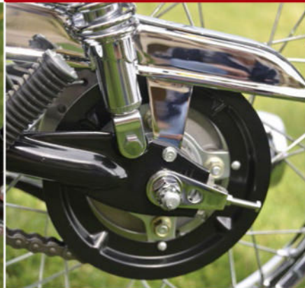
LEFT Pressed metal rear chain shrouds rarely survive the ravages of time. RIGHT Shroud helps to keep water off the pads.
