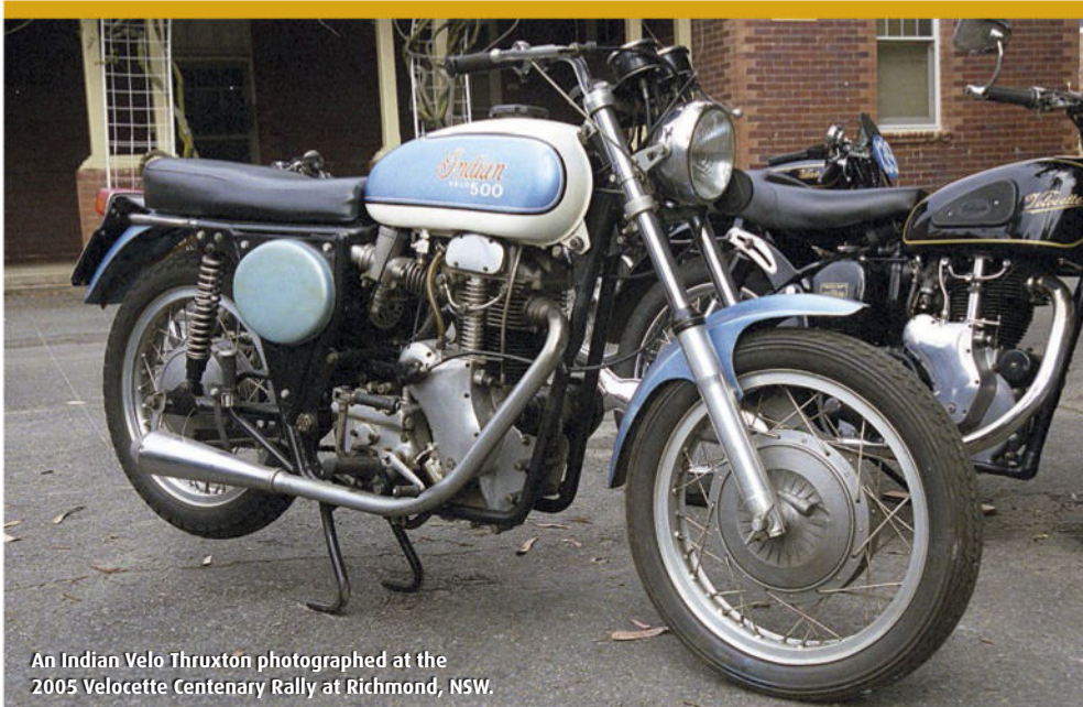
BELOW AND BOTTOM Two views of Alan Harper's Indian Velo – only the second one built and unusually fitted with magneto ignition.
