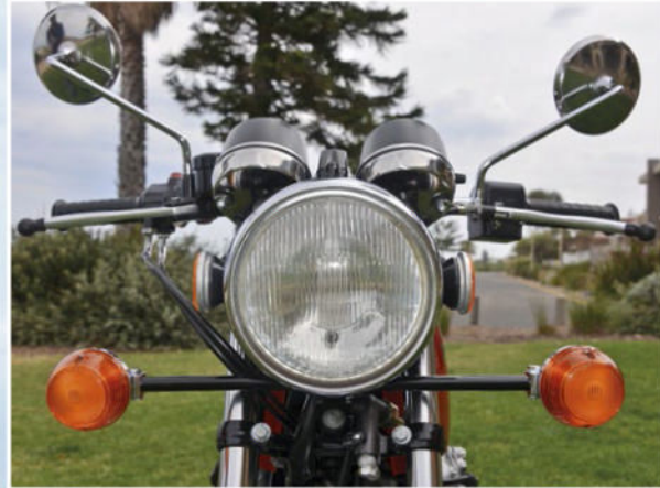
RIGHT Front indicators on the UK are wider apart than Australian delivery models.
