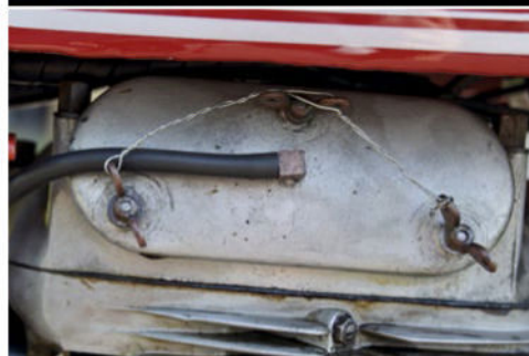
Standard oil tank was often replaced on scrambles bikes to allow an efficient air filter to be fitted.
