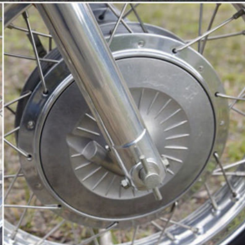
BELOW LEFT Rear chain guard mounts to the frame, hence the distance from the chain itself. Speedo drive is Smiths. BELOW RIGHT Grimeca front hub has the speedo drive flange cast in, but drive is actually taken via a Smiths unit from the rear hub.
