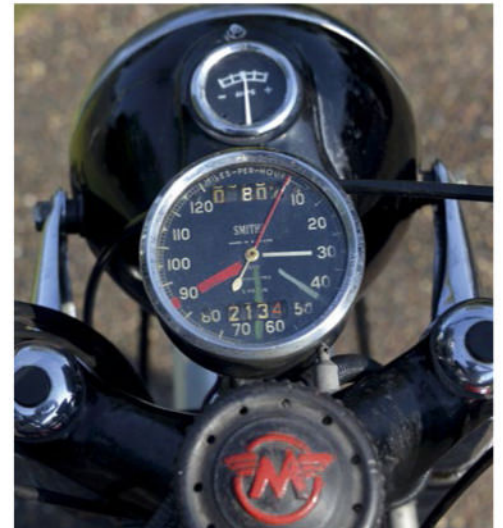
ABOVE Herb has painted 'gear change' points on the speedo dial. LEFT Exhaust pipe is routed over the footrest, which straddle the lower frame rails.
