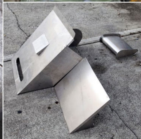
ABOVE The new chassis takes shape ABOVE RIGHT Seat base made by Bob Howle, who made the original fibreglass components. RIGHT Fairing and wing recreated in aluminium, as on the original.
