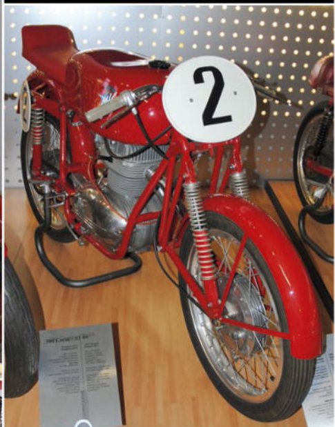
BELOW The boys' racer 175 - CSS/SV Squalo (Shark), derived from the road-going CSS. The 175cc chain-driven OHC single had a 5-speed gearbox and produced 19.8 hp at 8,800 rpm. As well as numerous road racing victories it also scored gold medals at the ISDT.
